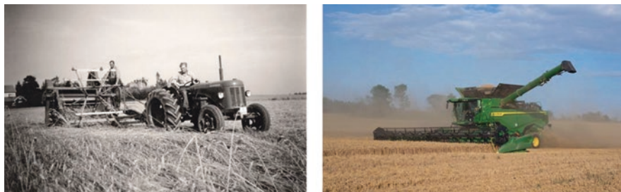
Fig. 15.1 One towed 5-foot header combine harvester (from 1954) that fills grain into sacks compared to the self-propelled X9 combine harvester with a 45-foot header and a 16,200-liter grain tank (from 2020)
