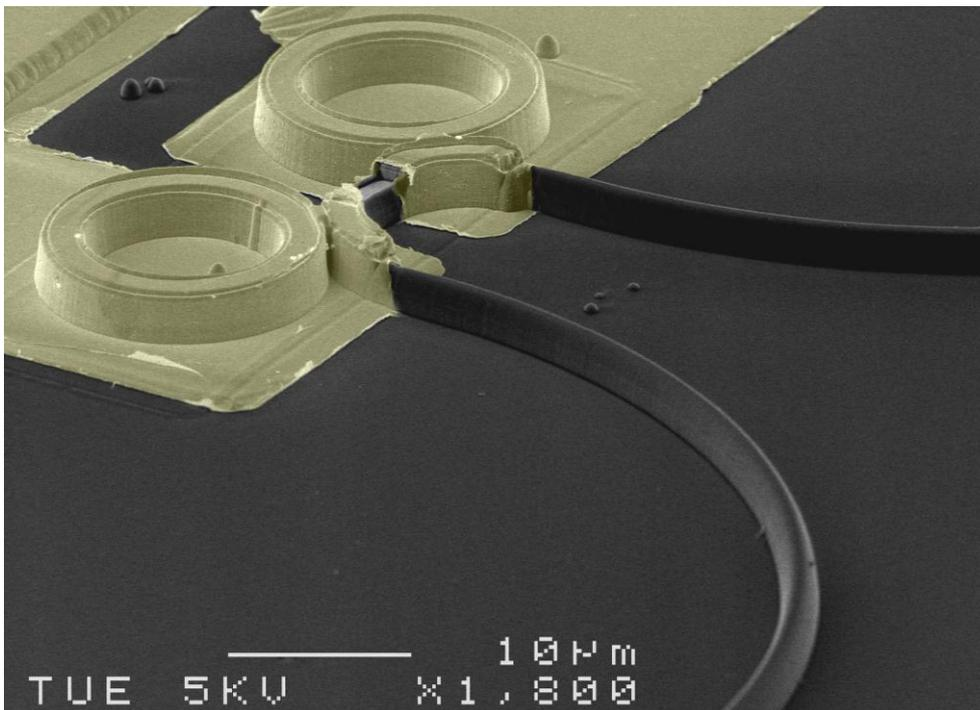
Fig. 1: Electron microscope picture of an optical flip-flop based on ring resonators with < 18 ps switching time. The device has been fabricated at TU/e<sup>10</sup> and occupies approximately  $60 \times 40 \mu\text{m}^2$ .
