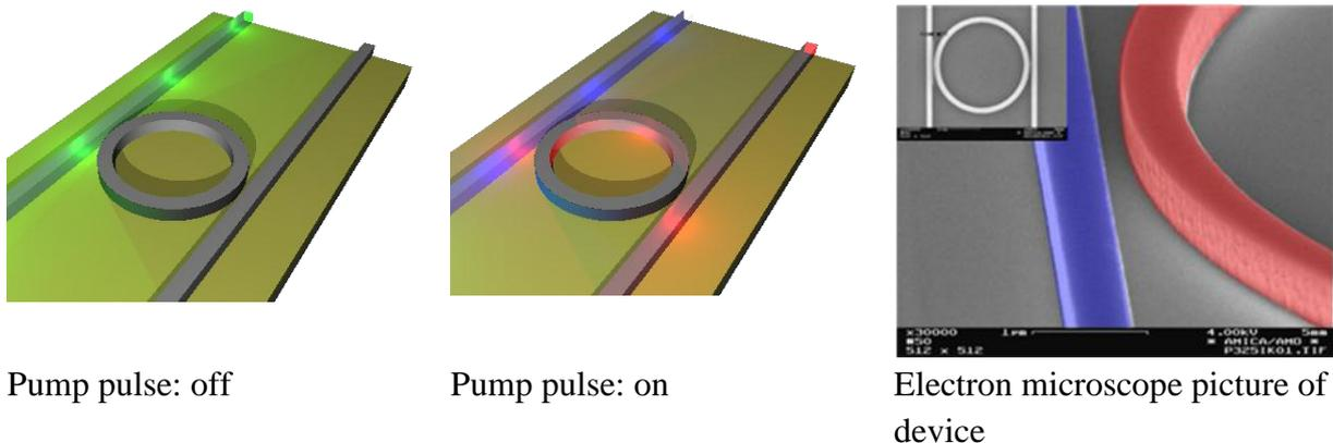
Fig. 2: Optical switch based on ring resonators with  $< 1$  ps switching time<sup>11</sup>. The device has been designed and characterized by UT in cooperation with the RWTH Aachen and occupies approximately  $8\,000 \times 15 \mu\text{m}^2$ .
