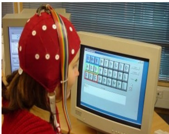
Figure 5. A person using a BCI based on motor imagery to select letters on a computer screen.
