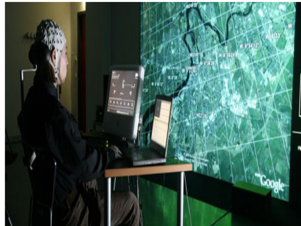
Figure 6. A person using a BCI based on visually evoked potentials to control Google Earth.
