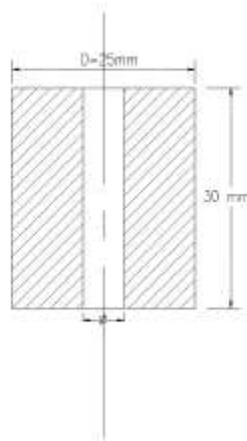
Fig.2 The work-piece.
