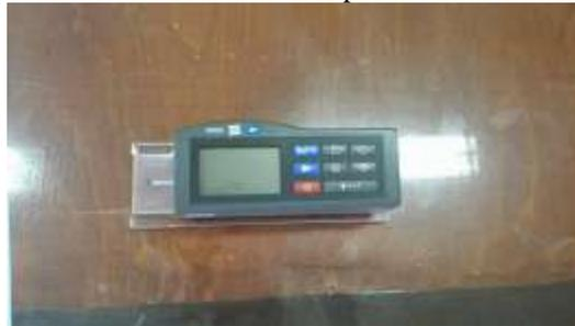
Fig.3. The surface roughness measurement device.
