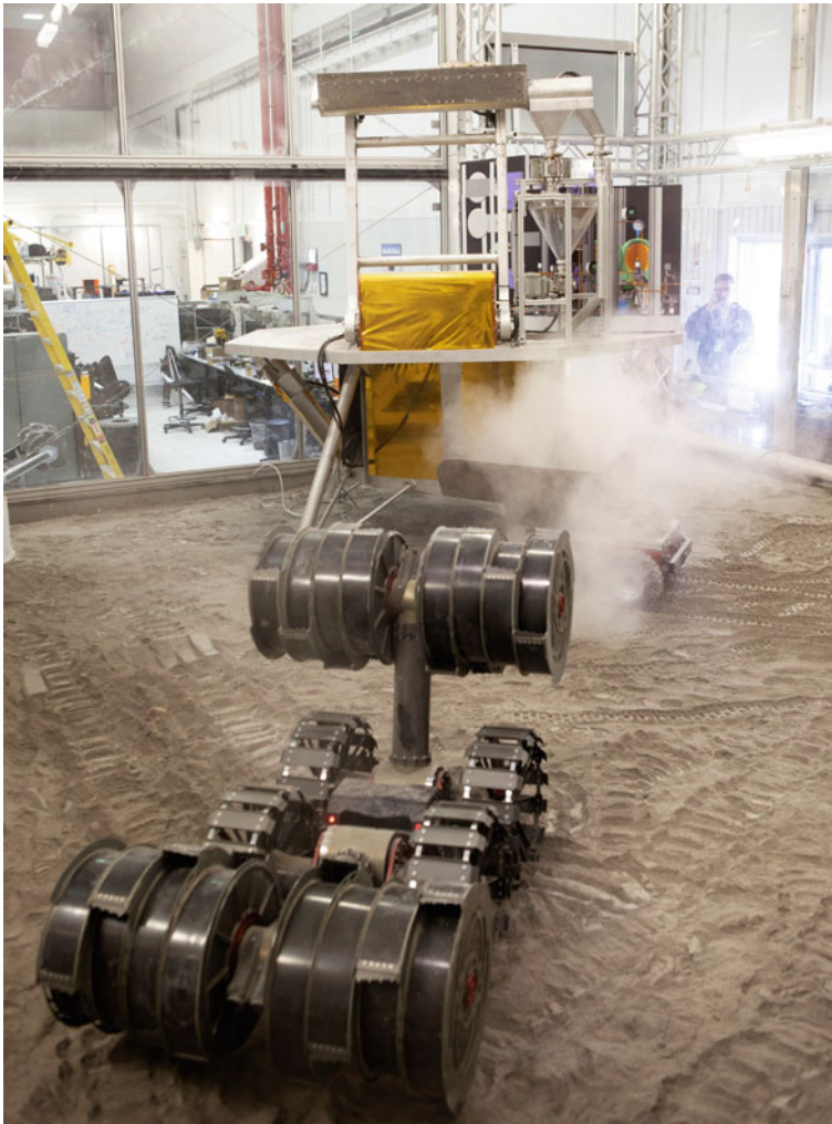
Fig. 4.6 NASA's Regolith Advanced Surface Systems Operations Robot (RASSOR) excavating simulated extraterrestrial soils. In-situ-resource-utilization strategies may be crucial for prolonged habitation on the lunar surface. Credit NASA
