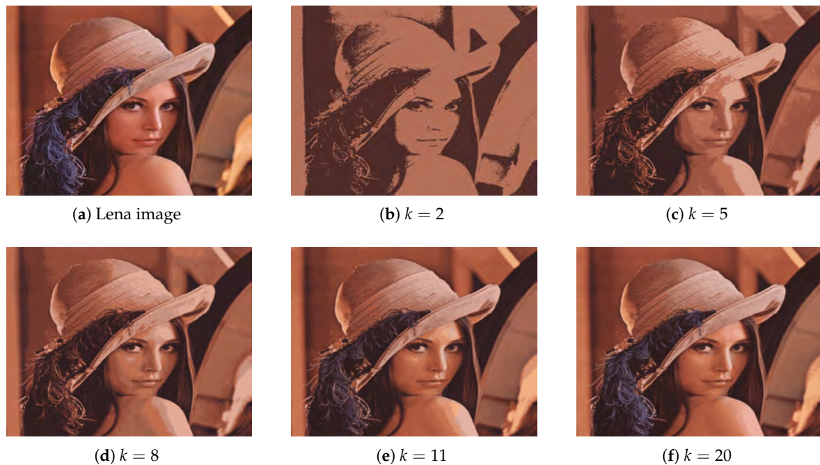
Figure 2. The image segmentation for the Lena image. (a) The original Lena image. (b–f) The clustering images when the number of clusters k = 2, 5, 8, 11 and 20 , respectively.
