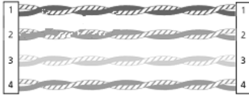
Figure 3. Assignment of Pairs in UTP cable.
