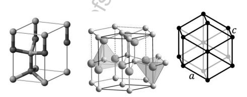
*Figure 4.2* Schematic representation of the principle of unit cells in X-ray crystallography with the example of the Wurtzite crystal structure (a mineral structure). Unit cells are the smallest repeating unit (left) from which to infer the general structural dimensions of the crystal (middle) and its geometric arrangement of the crystal (right). Unit cells act as an index. Images taken from Benjah-bmm27, 2007 (left); Solid State, 2008 (middle); Mayer, 2007 (right).
