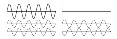
*Figure 4.5* Representation of different wave phases: in sync (left; from Haade, Wjh31) and out of sync (right; Quibik, 2010); the diffraction spots from in sync phases are stronger than those from out of sync waves.
