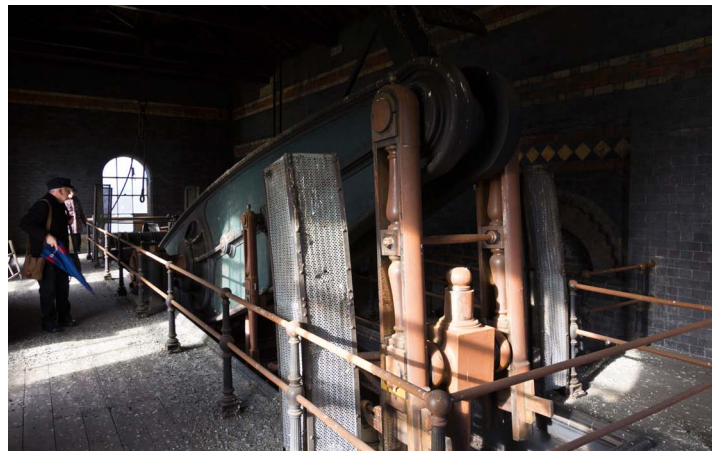
TOP: The Cornish engine had a 65-inch steam cylinder with a stroke of 9 feet. An elegant Tuscan arcade of three arches with fluted columns supported the bearing for the beam, which worked a 17.175 inch ram and 25.625 inch bucket pump.
