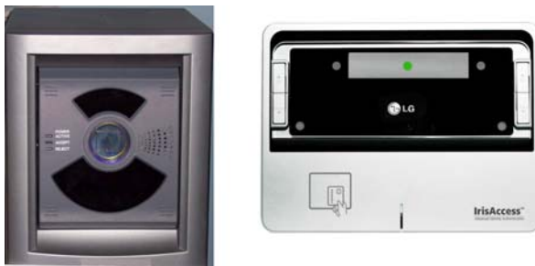
Fig. 7 LG 2200 ( left ) and LG 4000 ( right ) iris sensors. The 2200 system has near-IR LEDs at the top, lower left and lower right, and images one iris at a time. The 4000 has near-IR LEDs on the left and the right, and can image both irises at once
