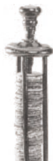
Figure 5. Two versions of Volta's pile, or column of electric generating elements. I The first featured a pile of silver and zinc disks, each separated from the adjoining pair by paper or cloth separators soaked in brine; the second featured a ring of cups filled with brine and connected by alternate strips of zinc and silver joined by metallic jumpers. The second form was an improvement over the first because the current tended to weaken as the brine in the separators dried out.
