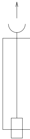
Figure 4: The Zombanimal Robot V1. The motor is denoted by the rectangular box at the tail end, the sensor by the half-circle on a stalk.
