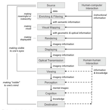
Fig. 1 A typical visualisation pipeline
