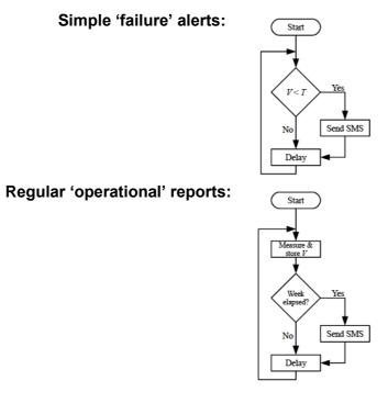
Fig. 3. Systems Diagrams for GSM enabled microprocessor remote monitor of battery voltage (recharged by dynamo on pump handle)
