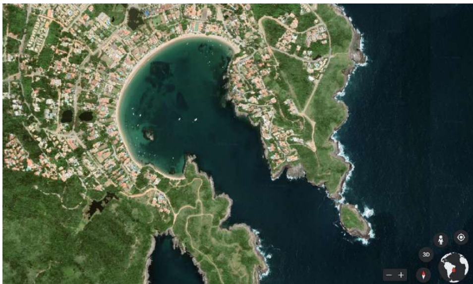
Fig. 3 – The shape of the Shell Beach (Praia das Conchas, Municipality of Cabo Frio) is controlled by the diffraction of waves on the hills, an example of the ecocentric value of balance. Source: Google Earth.
