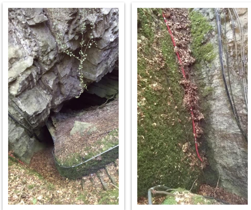
Photo VII.6: The staircase installed in the doline to access the cave (left). The Electrical Resistivity Tomography (ERT) profile of 48 electrodes starts vertically at the bottom next to the staircase (visible on the left) and progresses to the surface where it becomes horizontal (right). Source: ORB (Michel Van Camp).
