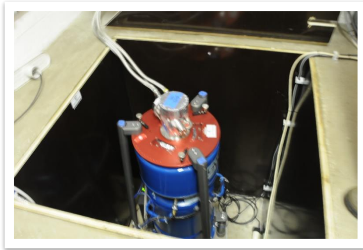
Photo VII.5: The relative superconducting gravimeter, with its shelter. Source: UCLouvain (Damien Delforge).
