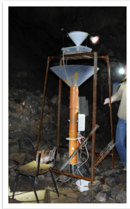
Photo VII.7: Drip discharge monitoring device within the cave (P1). Source: UCLouvain (Sebastien François).
