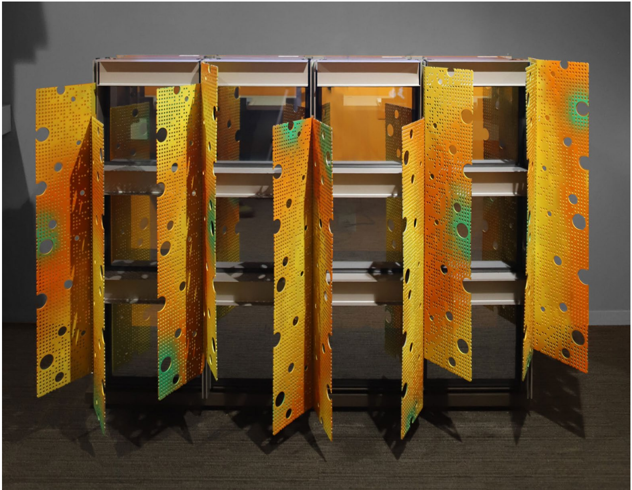
Figure 1: Example Construction by Group 2, custom laser cut steel sheet attached to standard extrusions. (Seminar Group 2: Chance Vidovic, Joel Dalzell, Brooklynne Irwin, Kalp Champaneri, Hunter Edmiston, 2022)
