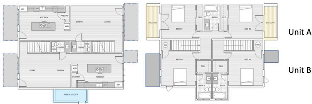
Figure 3: SOLEIL 1 st floor and 2 nd floor modules stacked and connected to stairway module on site to form 1-bedroom, 2-bedroom or 3-bedroom row house floor plans.(Garrison 2021)
