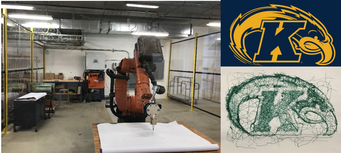
Figure 4: Robotic Portrait Sketching. (Left) Kuka KR60 Arm, (Right-Up) Input Image, (Right-Down) Sketch by Kuka Arm. Source: Authors
