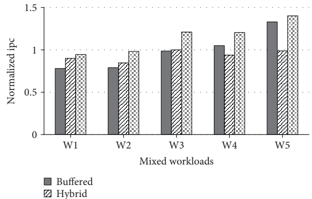
FIGURE 10: Normalized IPC of hybrid load with 64 threads.
