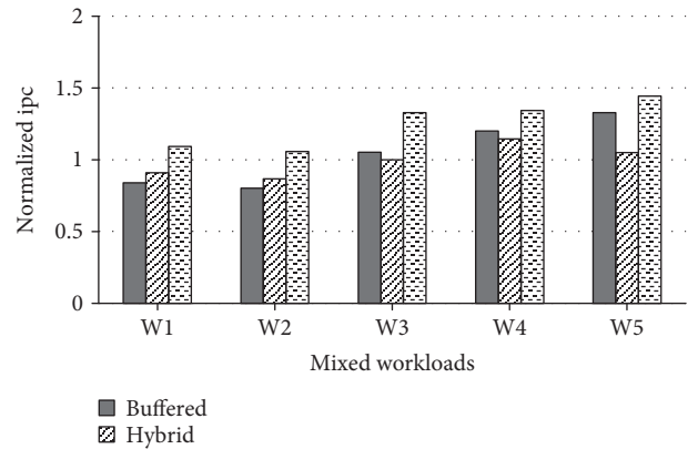
FIGURE 14: Normalized IPC of hybrid loads with 128 threads.
