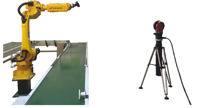
FIGURE 1: Experimental setup with ER20-C10 robot and Radian™ laser tracker.
