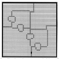
Figure 9. Wire crossing, allowing electron travel either south to north or west to east
