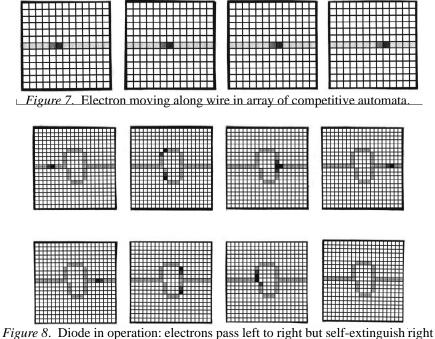
*Figure 8.* Diode in operation: electrons pass left to right but self-extinguish right to left
