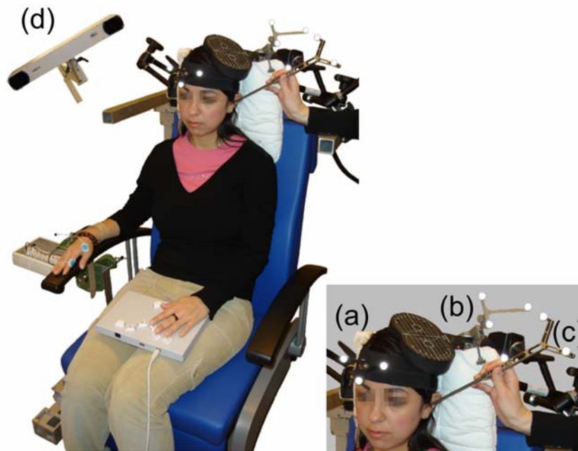
Fig.1 Neuronavigated TMS guided by frameless stereotaxy. A tracker with 3 passive spheres is attached to the headband of the subject (a), to the TMS coil (b), and fixed on a pointer (c). These dynamic reference systems provide online information about the location of the head and the coil in space. A camera system (d) detects the position of the dynamic reference systems and displays this information on a computer screen using navigation software for visual localization of the coil.
