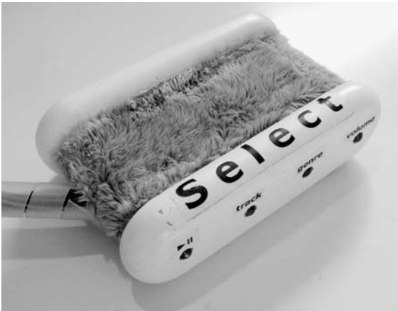
Fig. 1 Stroking on the select side of Puppy allows one to switch between functions (play/pause, track, genre, volume) and stroking on the opposite +/- side increases or decreases the chosen function. The direction of stroking and the character of the stroke (speed, area of touching and the length of the stroke) determine how the function is interpreted and executed
