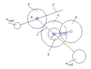
Figure 3: Complete shaking force and shaking moment balancing of an articulation dyad.
