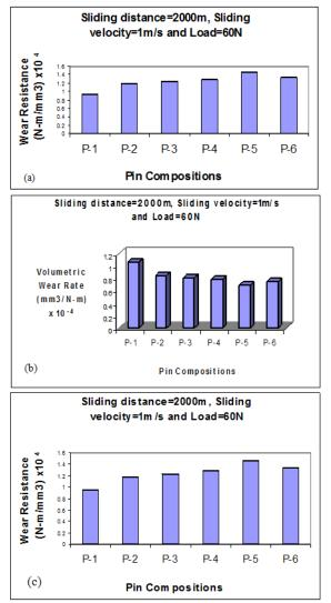
Figure 6 (a-c): Wear volume, wear rate and wear resistance of test specimens for sliding distance of 2000m, sliding velocity of 1m/s and at a normal load of 60N.
