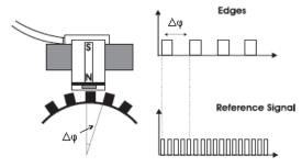
Figure 1 (b). Time measurement between two edges.
