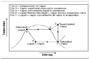
Figure 3: Temperature - Entropy diagram for ideal vapor compression cycle.
