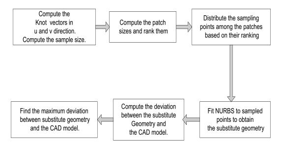
Figure 3: Patch size-based sampling flow diagram.
