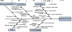
Figure 2: Cause and Effect Diagram for the Jamming Problem in the Cutting Machine.
