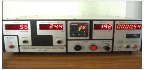
Figure 2: Controller of the wear and friction-testing machine.
