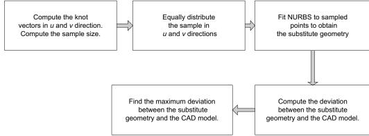
Figure 2: Flow diagram of the equiparametric sampling technique.
