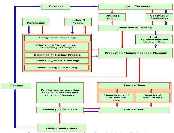
Figure 2: Standard sequence of operations for the manufacture of casting in the considered foundry.
