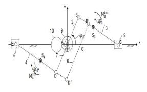
Figure 11: Self-balanced slider-crank system with an imagined articulation dyad B'D'E
