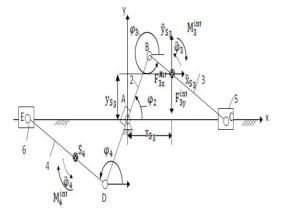
Figure 10: Self balanced slider - crank system.
