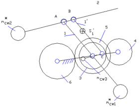
Figure 4: Complete shaking force and shaking moment balancing of an articulation dyad by gear nertia counterweights mounted on the base.
