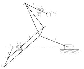
Figure 9: Balanced Atkinson engine mechanism.
