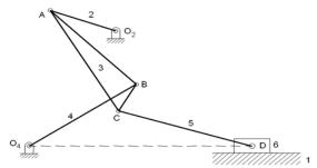
Figure 8: Atkinson engine mechanism.
