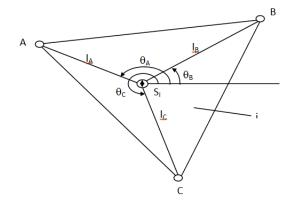
Figure 5: Dynamic substitution of the masses of the link by three rotational pairs.
