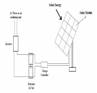
Figure 1: Solar system diagram.
