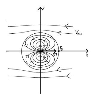
Figure 2. Flow structure of flow function (9).
