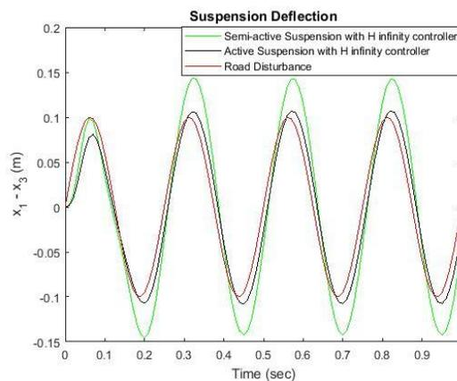
Figure 12: Suspension deflection for sine road disturbance
