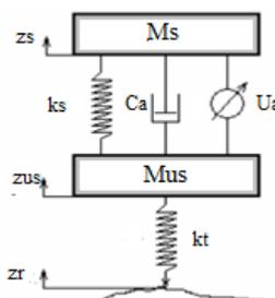
**Figure 1:** Quarter model of active suspension system.
