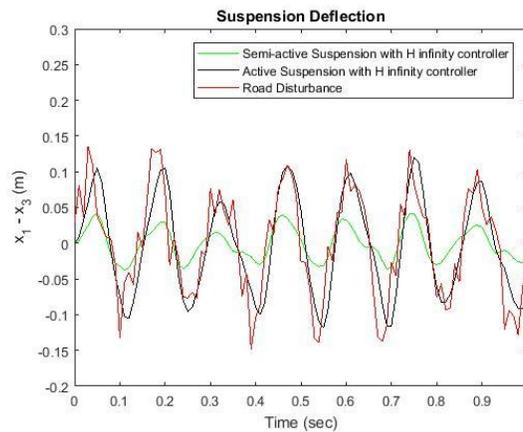
Figure 9: Suspension deflection for random road disturbance
