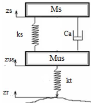
Figure 2: Quarter model of semi-active suspension system.
