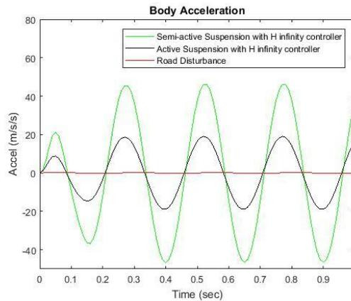
Figure 11: Body acceleration for sine road disturbance
