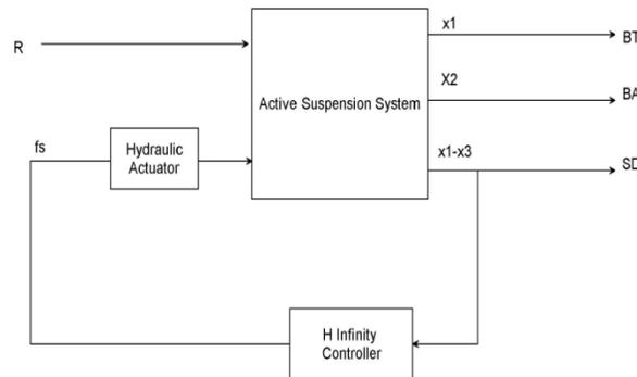
Figure 5: Active suspension system with  $H^\infty$  controller system block diagram
