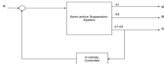
Figure 6: Semi-active suspension system with  $H^\infty$  controller system block diagram
