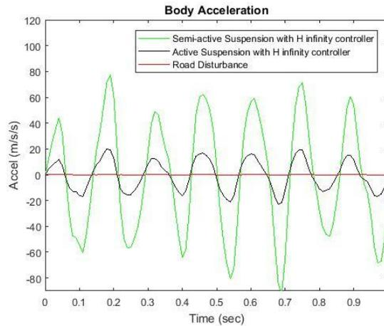
Figure 8: Body acceleration for random road disturbance
