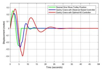
Fig. 10: Sine wave response of the trolley position comparison
