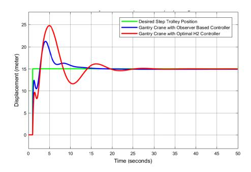
Fig. 5: Step response of the trolley position comparison
