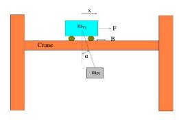
Fig. 1: Gantry crane system
