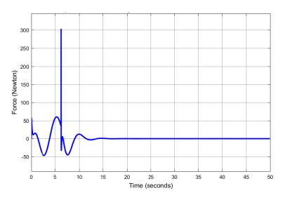
Fig. 12: Input force to the system with observer based controller
