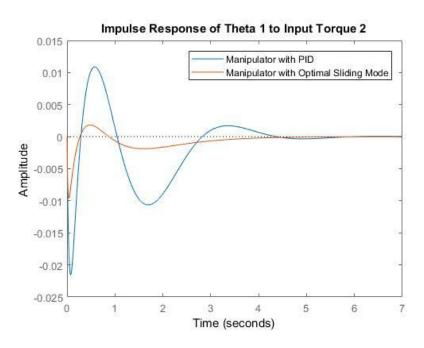
Figure 4 Impulse response of Theta 1 to Torque 2
