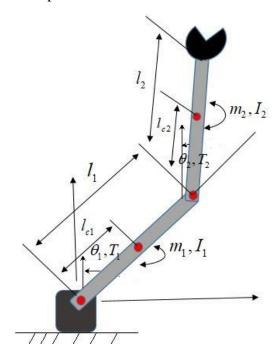
Figure 1 Vertically designed two link manipulator
