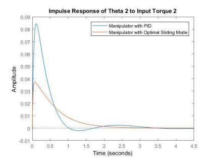
Figure 5 Impulse response of Theta 2 to Torque 2
