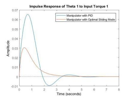
Figure 2 Impulse response of Theta 1 to Torque 1
