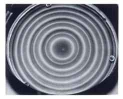
Fig. 3 Convection rolls of alternately larger and smaller section on a circular plate with a radial temperature gradient at the bottom (from Koschmieder 1993, p. 164)
