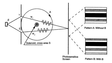
**Figure 2:** (From Liu 1994, p. 990).  $\Psi_1$  and  $\Psi_2$  represent the paths of electrons from the source S on the left to the screen on the right, and B represents the magnetic field within the solenoid. When field B is present, the interference pattern on the screen shifts from pattern A (above) to pattern B (below).
