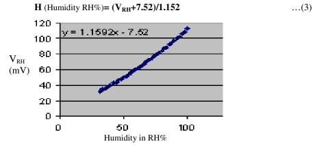
Figure 10: Graph of observed emf (mV) against applied humidity in RH%
