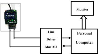
Figure 2.b: The schematics of the circuit of Base Station.
