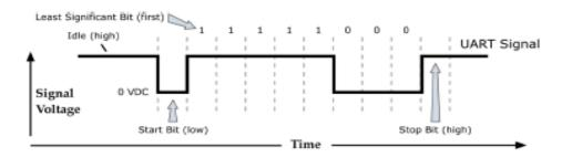
Figure 8. UART data packet 0x1F as transmitted through the RF module
