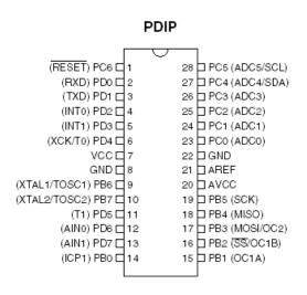
Fig.5: Pin description of AVR Atmega8L
