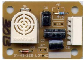
Figure 3: Humidity Sensor SY-HS-220
