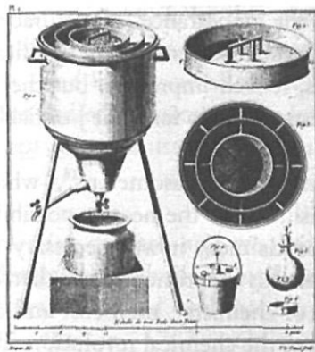
Figure 3: The ice calorimeter of Lavoisier and Laplace, in their «Mémoire sur la chaleur ... 1783», plate I.
