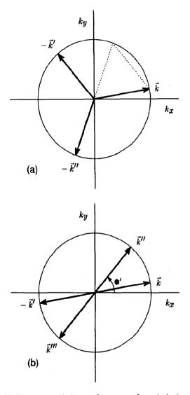
Fig. 3. Arrangement in k-space of wavevectors for modes having  $|\mathbf{k}| = k_c$  and satisfying (a)  $\delta_{k,k'+k'} = 1$  in the quadratic term of (7), and (b)  $\delta_{k,k'+k''} = 1$  in the cubic term. For the form of (7) to remain unchanged under symmetry operations of spatial translation and rotation the wavevectors must sum to zero.
