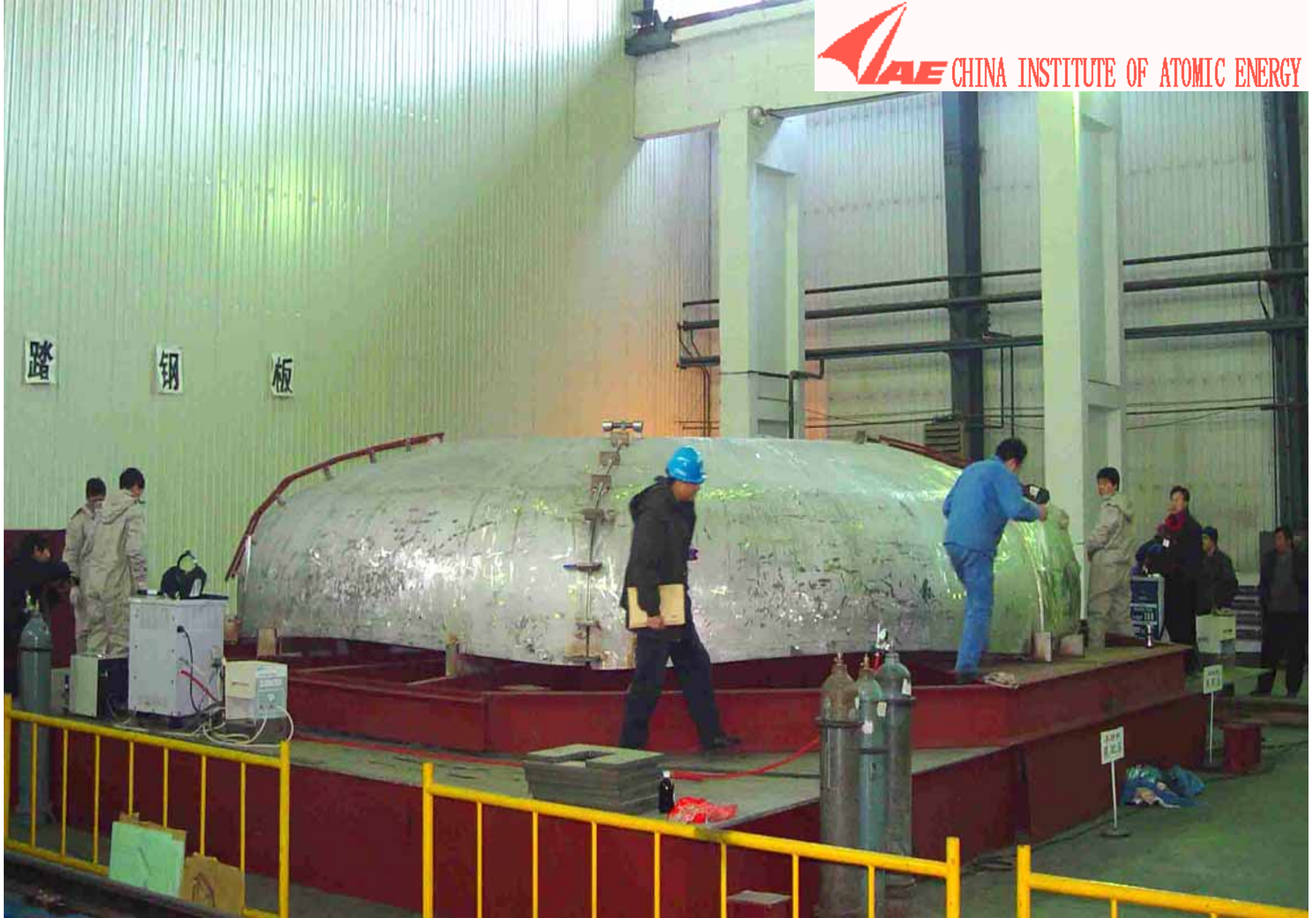
Reactor vessel closure under fabrication (in China)
