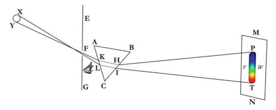
**Fig. 10** Newton's white synthesis in the style of his ally Desaguliers – here the experimenter looks *through prism ABC* at the spectrum PT. He sees a white image of the solar disk (Illustration by Ingo Nussbaumer, reproduced with his kind permission from Nussbaumer [RvI]:157; original drawing in Desaguliers [AoSE], Fig. 15)
