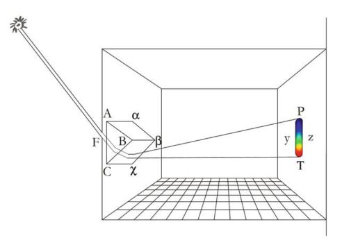
**Fig. 1** Newton discovers the heterogeneity of light. Lights rays are refracted by a prism  $ABC\alpha\beta\chi$  (*left*). In the dark chamber on the right, Newton catches his well-known spectrum  $S_N$  between the two poles P and T. The light rays that are redirected from their path the furthest are *blue*. They can be seen in the upper part of the spectrum (Redrawn by Ingo Nussbaumer; the original is in Newton's notebook, reprinted in Newton [UFVo]:3)
