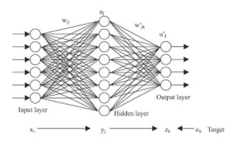
Fig. 7 Artificial Neural Networks model
