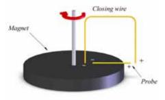
Figure 1 – Basic homopolar setup
