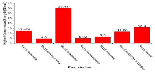
Figure 5. Highest compressive strength of previous studies on brick incorporated with plastic waste aggregate.
