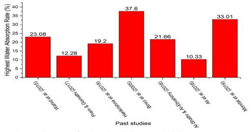
Figure 4. Highest water absorption rate of previous studies on bricks incorporated with plastic waste aggregate.
