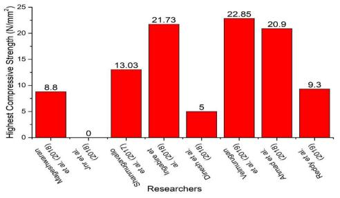
Figure 7. Highest compressive strength of paving block utilised plastic waste as aggregate based on previous studies.
