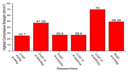
Figure 8. Highest compressive strength of paving block incorporated with plastic waste aggregate.
