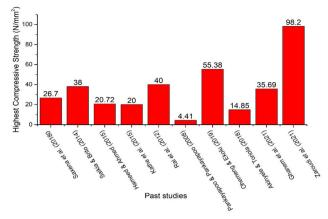
Figure 1. Highest compressive strength of plastic waste included construction based on previous studies.
