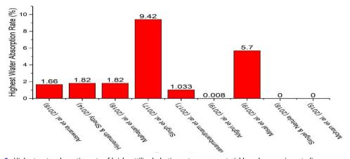
Figure 2. Highest water absorption rate of bricks uttilised plastic waste as raw material based on previous studies.
