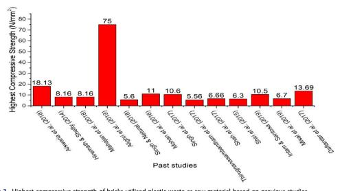
Figure 3. Highest compressive strength of bricks utilised plastic waste as raw material based on previous studies.
