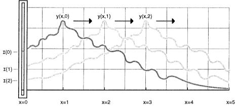
Figure 4. Retarded solution of one dimensional wave equation.
