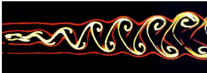
Figure 1: Wake behind a cylinder, seen from above
