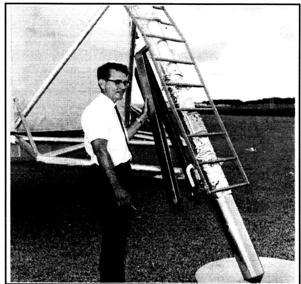
Fig. 4. Dave McCraw, NASA Manned Spacecraft Center Technical Services Deputy Division Chief, demonstrates the removal of the flag shroud from the Lunar Module ladder. He holds the "pip" pin in his right hand (NASA photograph S69-38755).
