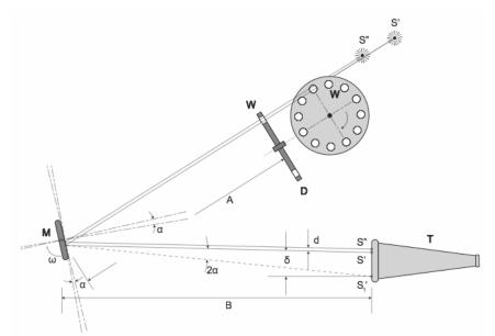
Let us choose two celestial bodies S' and S" as two possible sources of luminous beams at velocities c' and c''. These bodies must be visually close enough in order to be simultaneously focused by the telescope T through the rotating mirror M and the window W. In addition, the selected celestial bodies must have quite different radial velocities R' and R", in order to maximize the sought-after result.
