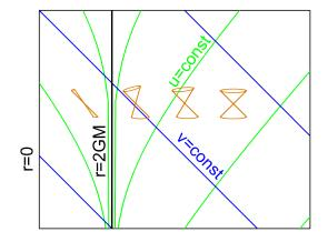
Figure 1. Space-time diagram in Eddington-Finkelstein coordinates showing the light cones close to and inside a black hole. Here,  $r = 2GM = r_S$  is the Schwarzschild radius where the event horizon is located (units c = 1).
