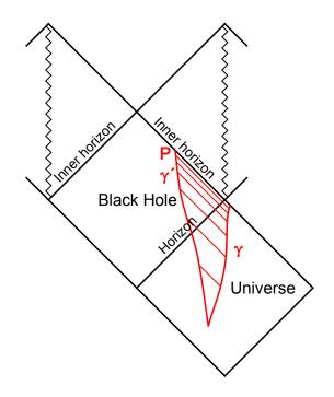
Figure 4. Carter-Penrose diagram of a Kerr black hole. The trajectories of two physical systems are indicated:  $\gamma$  remains in the exterior space-time for an infinite amount of time, whereas  $\gamma'$  falls into the black hole. In the time it takes the latter to reach the inner horizon, the former arrives to the conformal infinity. The lines that connect both trajectories represent signals sent from  $\gamma$  to  $\gamma'$ .
