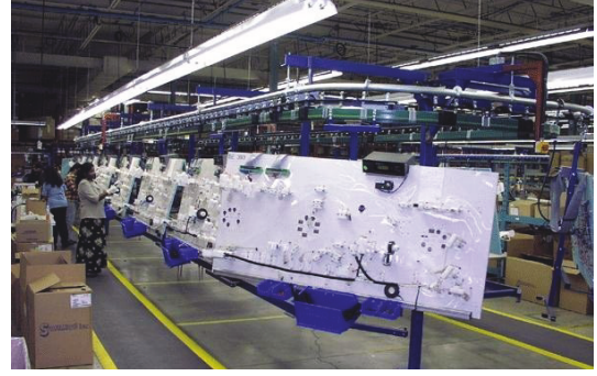
FIGURE 13: The wire-harness assembly pace conveyor [62]. The conveyor (often referred to as rotary) contains assembly tables consisting of connector and clip fixtures.
