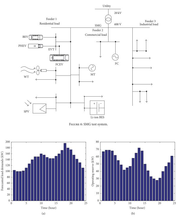
FIGURE 7: (a) Forecasted load demand and (b) operating reserve capacity.
