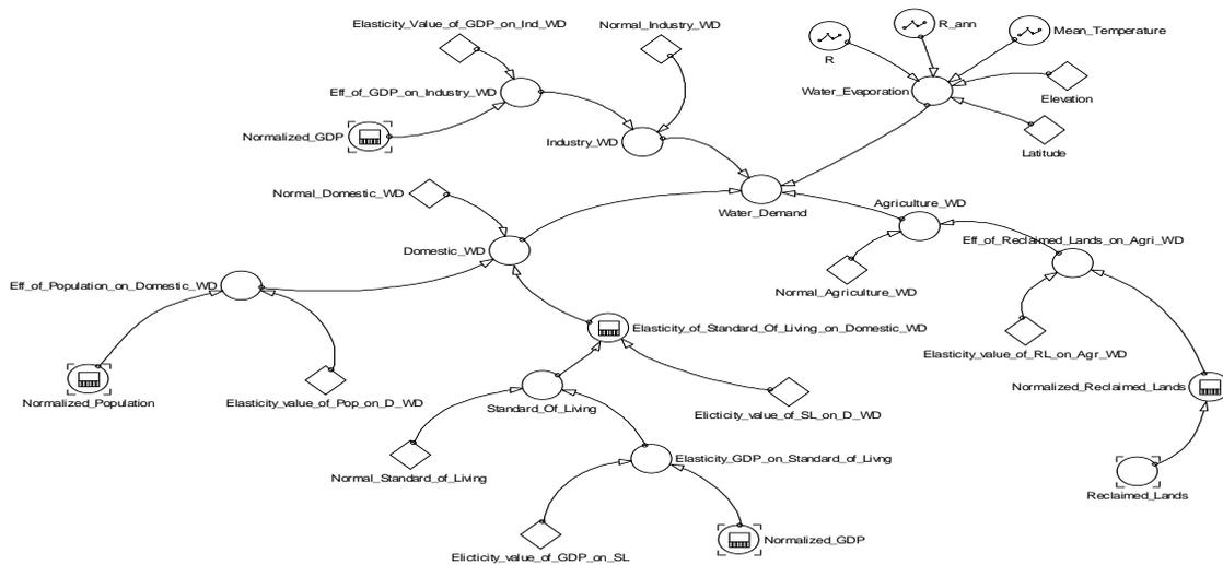
Fig. 6. Stock and flow diagram of water demand
