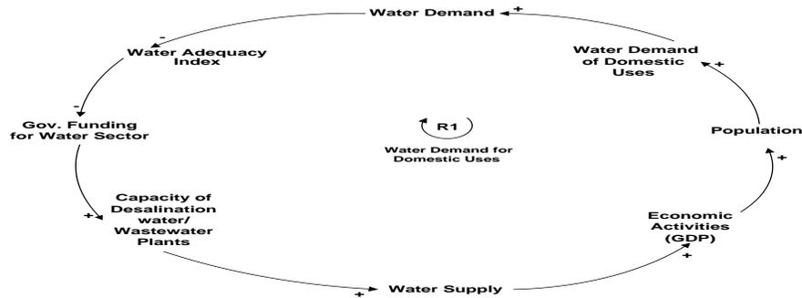
Fig. 5. Water demand for domestic uses loop
