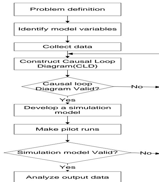
**Fig. 4.** Flowchart of building a simulation model.
