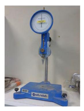
Fig. 13. Laboratory penetration cone.
