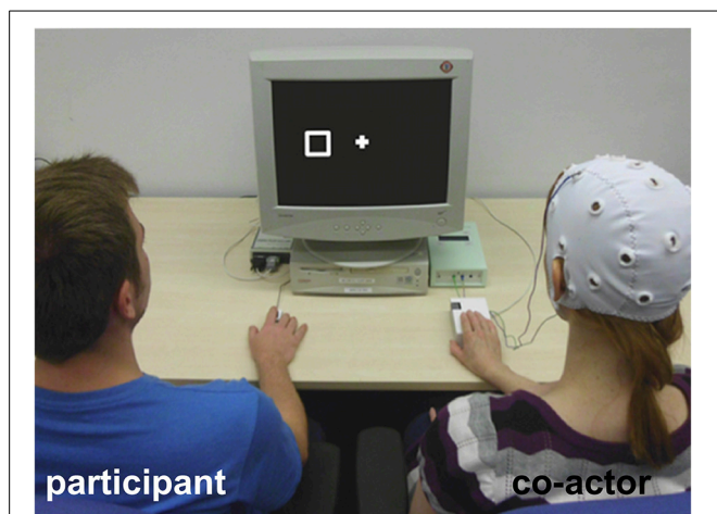
FIGURE 3 | Experimental setup used in Experiment 2. The participant (left side) shared a joint go/nogo Simon task with a co-actor (confederate, right side) wearing an EEG cap with electrodes attached to the motor cortex, and placing the finger underneath the moving part of a response device. The participant was either told that the confederate intentionally controlled the response button via a BCI so that the causal relationship between co-actor and action effect was not perceivable (agency-/intentionality+ condition) or that the response button was controlled by the computer (agency-/intentionality- condition). As the same response button was used for the co-actor in the agency-/intentionality+ and the agency-/intentionality- condition, the setup shown on the picture applies to both conditions.
