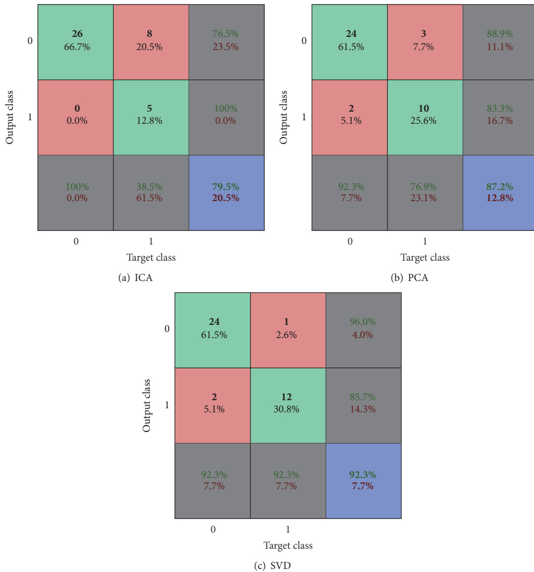
FIGURE 19: Confusion matrices of classification using the optimized Naive-Bayes for ICA, PCA, and SVD data reduction techniques.
