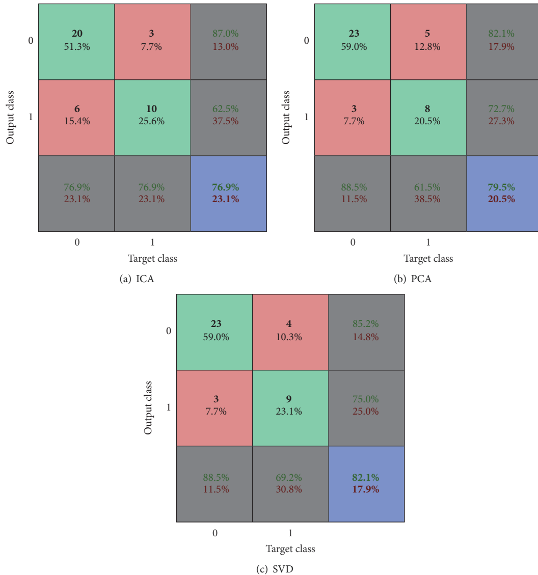
FIGURE 16: Confusion matrices of classification using the Gaussian Naive-Bayes for ICA, PCA, and SVD data reduction techniques.
