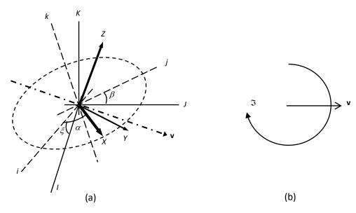
Figure 9A.3. (a) Relationship between angles and axes for the equation of motion. The direction of **v** in this diagram is arbitrary. The *XYZ* triad is arranged to agree with the flipped triple-triad (proton) of Figure 5.12b. The -X - Y - Z triad is omitted for clarity but is included in Figure 9A.2 (dotted axes). (b) Direction of motion of  $\Im$  in relation to the particle velocity **v**.
