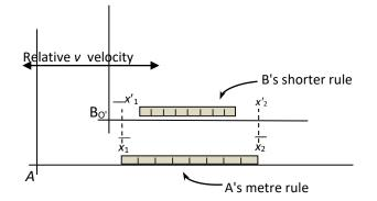
Figure 9.13. B takes a photograph of A's metre rule. Due to the relative motion, B's metre rule will be shorter than A's metre rule. In terms of his rule he therefore measures  $\Delta x' > \Delta x$ . The inverse condition with A travelling past B and photographing a metre rule placed on B's *X*-axis would show the equivalence of the two frames for this physical action.
