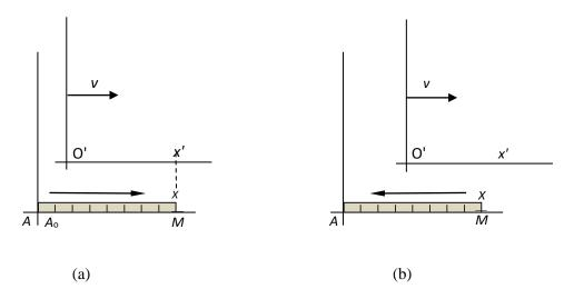
Figure 9.11 Given two observers A and O' at the origins  $A_0$  and O' of their respective frames of reference A and O', a metre rule (or rod) of length x is placed along the x-axis of the A frame with one end at  $A_0$ . A photon of light (lower arrow) is dispatched from A at time  $t_0$  to a mirror M and reflected back to A. O' moves with velocity v to the right in relation to A. In the right hand diagram (b) the wave reflects off M and returns to A.
