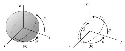
Figure 6.3 (a,b) Description of a ball rotating in the  $\dot{\alpha}$  and  $\dot{\beta}$  directions in the *IJ* and *JK* planes respectively with overall rotation  $\dot{\theta}$  (replaced by  $\dot{\phi}$  as in Figure 6.2) along the dashed line.
