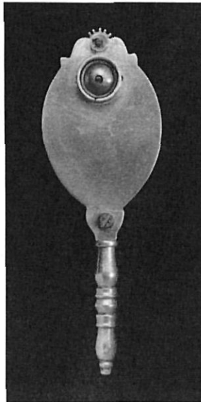
Fig I.9 Full plate Huygens-type simple microscope not signed. Courtesy of Sotheby's London
