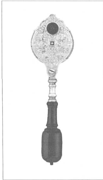
Fig I.12 Full plate Huygens-type simple microscope by John Marshall, London. Courtesy of Sotheby's London
